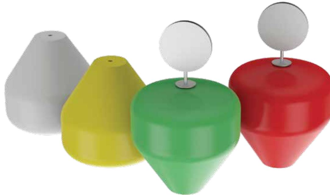
Tritonbuoys has developed a diverse selection of navigation buoys that adhere to rigorous quality standards and boast a proven track record of reliability. Each buoy is crafted from premium UV-stabilized virgin polyethylene and filled with closed-cell polyurethane to prevent water ingress if the outer layer is damaged. This design ensures exceptional performance and long-lasting durability.
